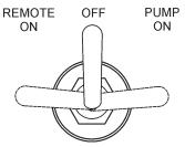
Figure 21. Pumping Control Switch (OFF)
